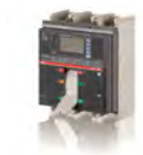
T7H 1000 PR332/P LSIRc In=1000A 3p F F
